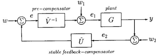
Fig. 2.2. Feedback system with external inputs.
