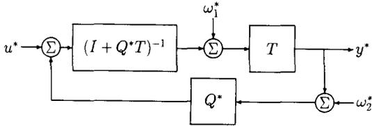
Fig. 3.6. The class of (bounded-input) stabilizers for  $T$ .
