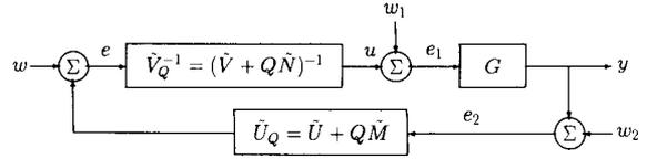
Fig. 2.3. The class of all (bounded-input) stabilizers of  $G$ .
