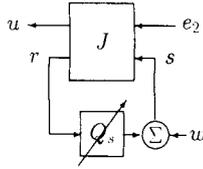
Fig. 3.3. Re-configuration of the controller  $K_{Q_s}$ .
