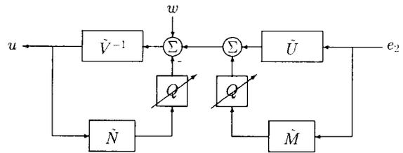
Fig. 3.1. The controller  $K_Q$ .
