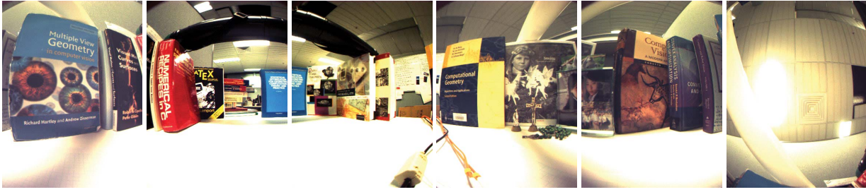
Figure 11. Six images captured at each camera of LadyBug. Five cameras (camera id 0 to 4) are placed to look horizontally view, and the last one (camera id 5) is located for a top view (From left to right order). There are only small overlapped fields of view across cameras.
