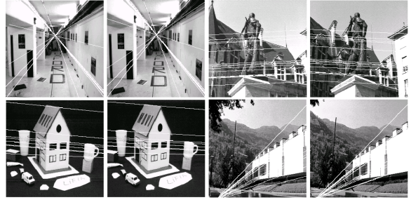
Figure 3. Some standard test images with estimated epipolar lines (using the 5-pt algorithm) superimposed on.
