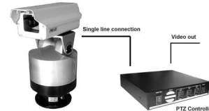
Figure 1. A typical surveillance PTZ camera system setup.
