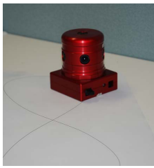
Figure 8. Left: our experiment setup. A ladybug camera is moving along a plotted planar curve; Right: spatial configurations of its six camera units.
