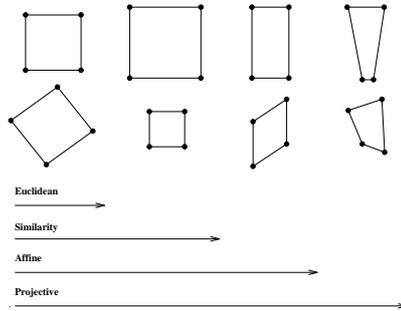
Figure 3: THIS FIGURE WILL BE INCLUDED IN THE TABLE. The hierarchy of plane to plane transformations. These range from Euclidean, where only translations and rotations occur, to projective where the square can be transformed to any arbitrary quadrilateral (provided no three points are collinear). Typical invariants to these transformations are given in table 1.
