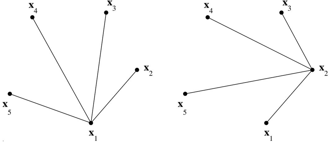
Figure 4: Five points on the plane have two functionally independent projective invariants. These can be expressed as the cross ratio of four lines from a base point to the other four points.
