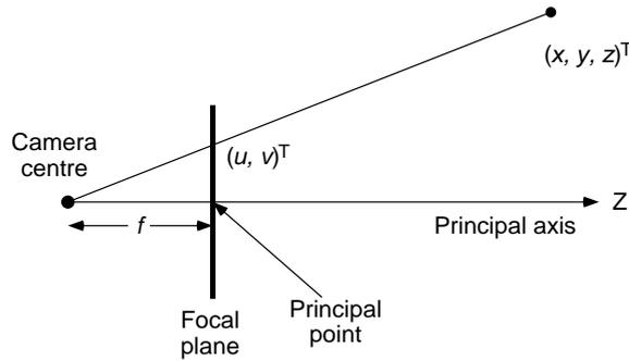
Figure 1: *Pinhole camera geometry*
