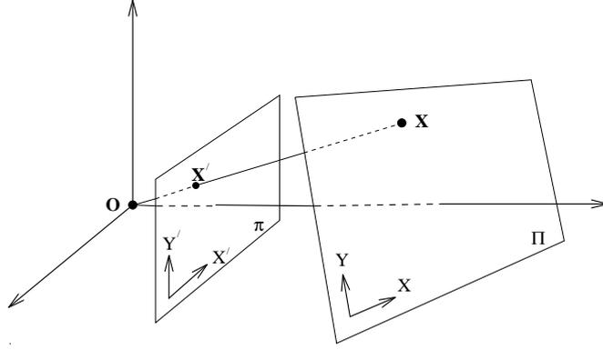
Figure 2: A perspective transformation between two planes: a world plane,  $\Pi$ , and an image plane,  $\pi$ , with optical center  $\mathbf{O}$ . The projection is modelled as a linear transformation,  $\mathbf{X}' = \mathbf{T}\mathbf{X}$ , on homogeneous point coordinates.
