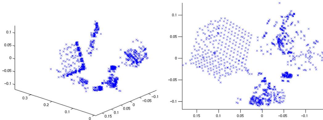
**Figure 3.** Top view and side view of the reconstructed scene points as computed using the square-pixel constraint. These results show that the Euclidean structure of the scene is well captured, as evidenced by the square shape of the calibration cube shown in the scene. The reconstruction results using only the zero-skew constraint were less satisfactory as can be expected.
