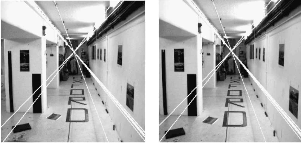
Figure 4: Corridor Scene In the corridor scene the epipoles are right in the image.
