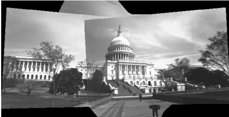
Figure 1: A composite image constructed from five different views of the Capitol. The composite image shows very clearly the projective distortion necessary for matching the images. Analysis of this projective distortion provides the basis for the calibration algorithm.
