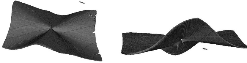
Figure 6: Shape of the possible rotations for 3 point correspondences. The space of possible rotations forms a surface in 3-dimensional rotation space.
