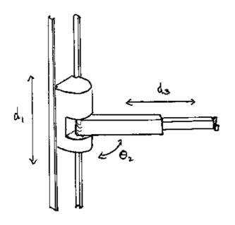
The home position for the robot (with  $d_1 = 0$ ,  $\theta_2 = 0$ ,  $d_3 = 1m$ ) has the base of the robot on the ground, the arm pointing straight out and the end effector one metre from the vertical axis. (Note that joint limits prevent  $d_3 = 0$ .) The revolute joint  $\theta_2$  is measured positive in a counter-clockwise direction from home.
