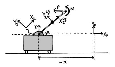
In the modelling of the dynamics an external force and torque (F, N) is generated at the handle of the walking stick by the client.
