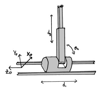
The robot is mounted sideways on the tunnel wall (as shown in the figure) and inserts samples into the slots cut into the opposing wall. The base frame is oriented with the  $X_0$  axis horizontal to the floor of the tunnel, the  $Y_0$  axis is in the vertical positive direction and  $Z_0$  lies along the axis of the tunnel. The base cart of the robot weighs 20kg. The inner and outer arm links are both 1m in
