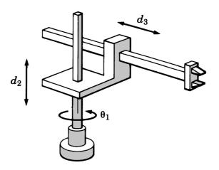
The Denavit-Hartenberg parameters for this robot are
