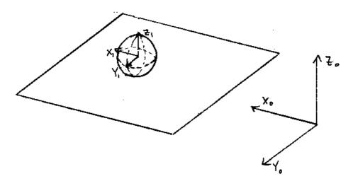
The position of the ball is irrelevant, only its attitude is of interest. The ball can be rolled forward in the  $X_0$  direction or sideways in the  $Y_0$  direction.
