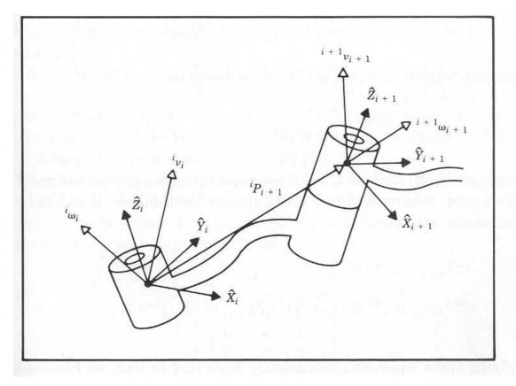
Remember that linear velocity is associated with a point and angular velocity with a body (frame); hence the linear velocity of a link means the linear velocity of the origin of the link frame and the angular velocity of a link means the angular velocity of the link frame.
