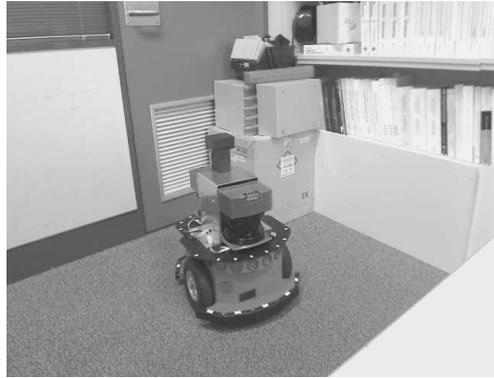
Fig. 1. Experiments: Pioneer DX3 Robot roaming in part of our laboratory
