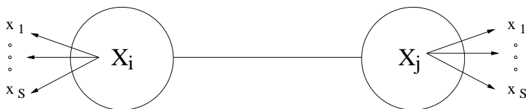
Fig. 2. Local “kernel” structure of the Graphical Model. Each random variable can assume S possible realizations, so that the sample space for two connected random variables has S^2 elements.
