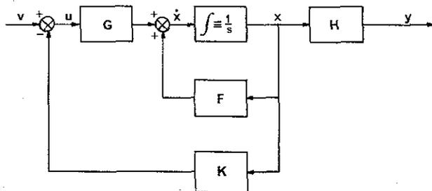
Figure 3.—System with state-variable feedback.
