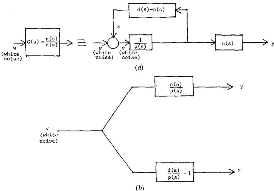
Figure 1. Justification of the all-pass factorization.
