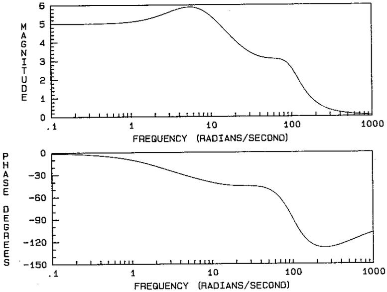
Figure 7. Example 2: original system:  $G(s) = \frac{20\,000}{s^2 + 100s + 100\,000} + \frac{50}{s + 10} + \frac{10}{s - 5}$
