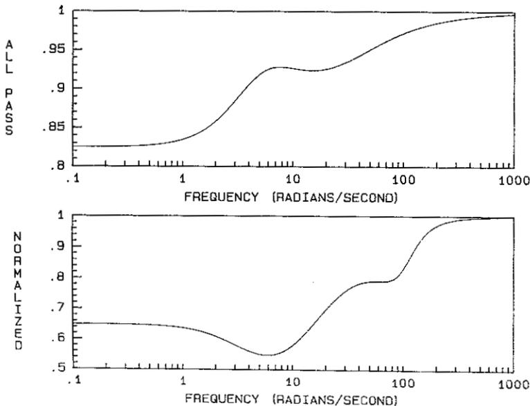
Figure 9. Example 2: preservation of unstable pole count in factorization methods:
