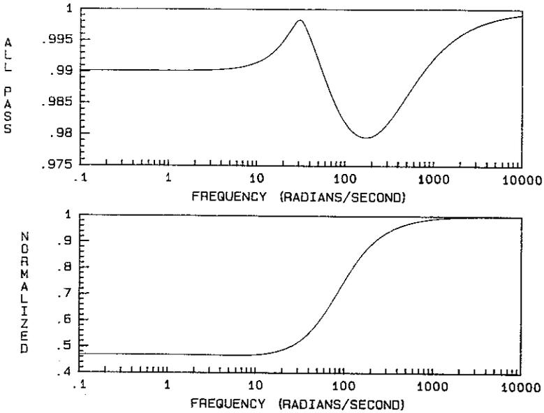
Figure 5. Example 1: preservation of unstable pole count in factorization methods:
