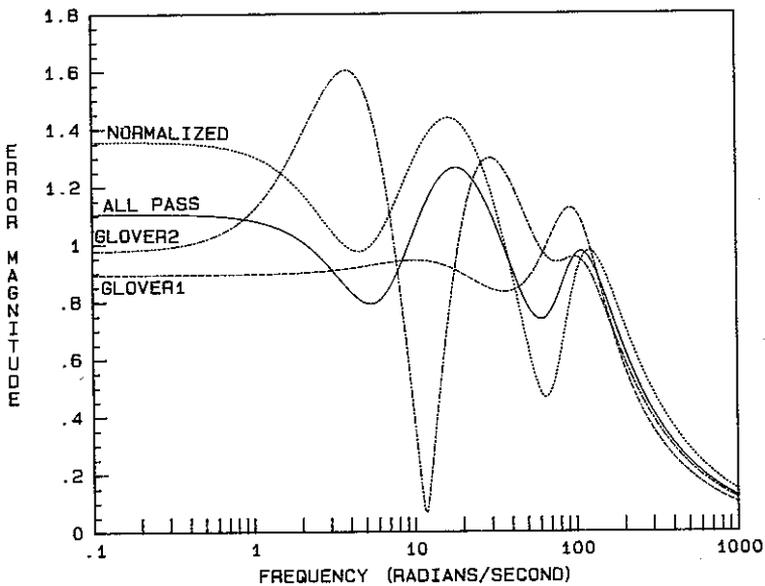
Figure 8. Example 2: comparison of approximation methods error magnitude:  $|G(j\omega) - \hat{G}(j\omega)|$ .
