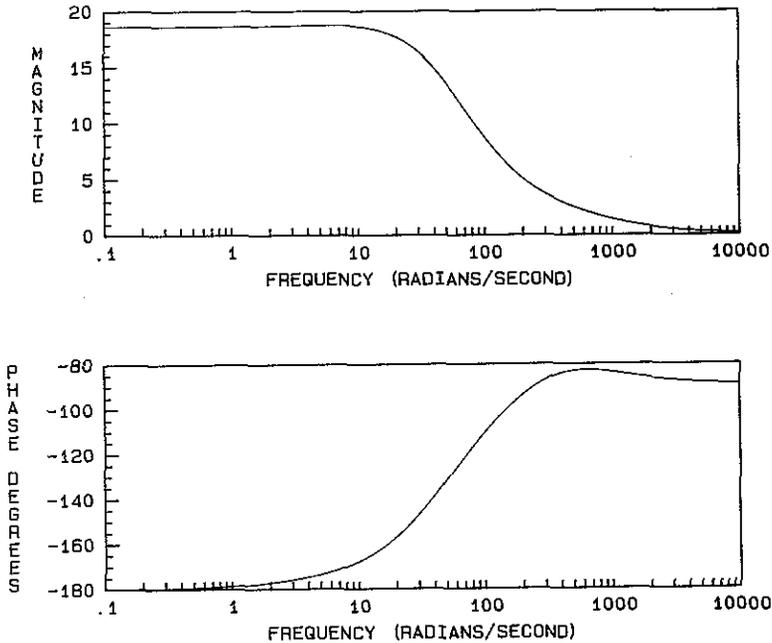
Figure 3. Example 1: original system  $G(s) = \frac{500s + 3400}{s^2 + 505s + 2500} + \frac{1000}{s - 50}$ .
