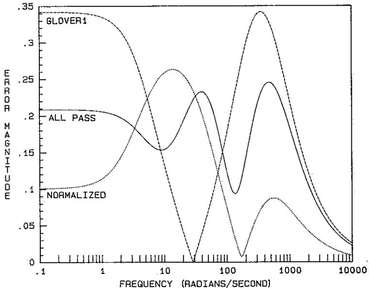
Figure 4. Example 1: comparison of approximation methods, error magnitude:  $\|G(j\omega) - \hat{G}(j\omega)\|$ .
