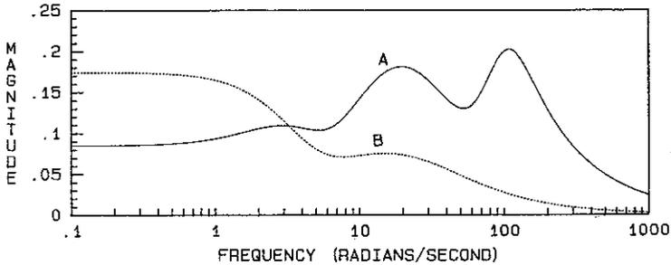
Figure 10. Example 2: factor error in the all-pass approximation:
