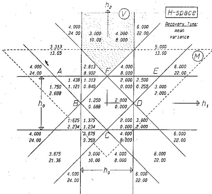
**FIGURE 2:** The Channel Parameter Space for  $N=2$ . The 29 Polytopes are bounded by the solid lines, the Minimum Phase Region by a dashed triangle. Numbers within polytopes give Mean (top) and Variance (bottom) of the Recovery Time. Uniform Distribution values on the left, Single Noise Induced Error Distribution on the right.
