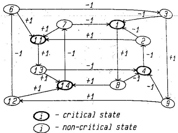
**FIGURE 3:** Pathological Sequence State Transition Diagram for Polytope  $V$ .
