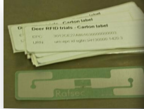
Figure 5.9 - UHF RFID ta... used on cartons Figure 5.9, Figure 5.10 and... in the boning room and mo... for loading the shipping cor...
