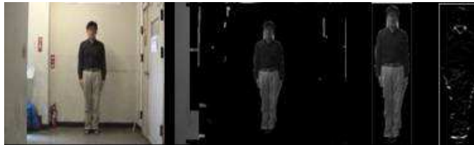
Figure 12: Background subtraction method: (from left to right) original image, background subtracted image, segmented image and Sobel edge image.
