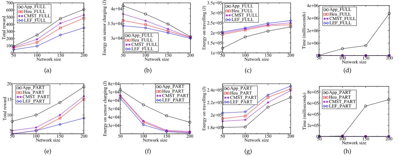
Fig. 3. The performance of different algorithms by varying network sizes. (a) The total reward. (b) The total energy on sensor charging. (c) The total energy on travelling. (d) The running times of algorithms. (e) The total reward. (f) The total energy on sensor charging. (g) The total energy on spent travelling. (h) The running times of algorithms.
