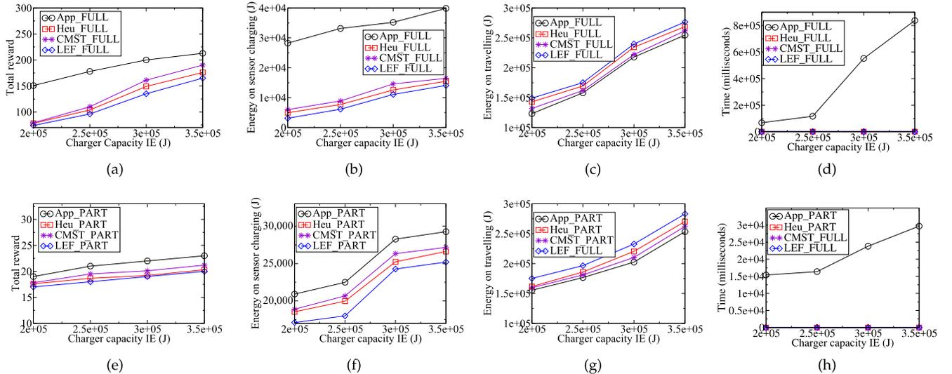
Fig. 4. Impacts of the energy capacity  $IE$  of the mobile charger on the performance of different algorithms. (a) The total reward. (b) The total energy on sensor charging. (c) The total energy on travelling. (d) The running times of algorithms. (e) The total reward. (f) The total energy on sensor charging. (g) The total energy on travelling. (h) The running times of algorithms.
