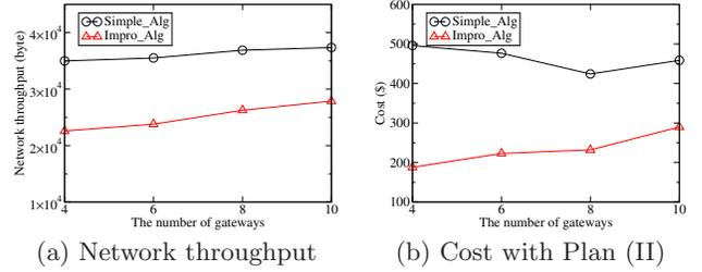
**Figure 4:** Impact of  $K$  on the network performance when  $n = 200$ ,  $p_e \in [0.1, 1]$  for each link  $e \in E$ , and Plan (II) is adopted.
