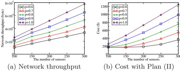
**Figure 2:** Impact of link reliability  $p$  on the network performance when  $K = 6$  and Plan (II) is adopted.
