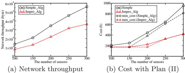
**Figure 3:** Performance of different algorithms when  $K = 6$ ,  $p_e \in [0.1, 1]$  for each link  $e \in E$ , and Plan (II) is adopted.
