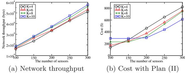
**Figure 1:** Impact of  $K$  on the network performance when  $p = 0.8$  and Plan (II) is adopted.
