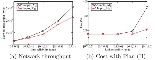
**Figure 5:** Impact of the range of link reliability on the network performance when  $K = 6$ ,  $n = 200$ , and Plan (II) is adopted.
