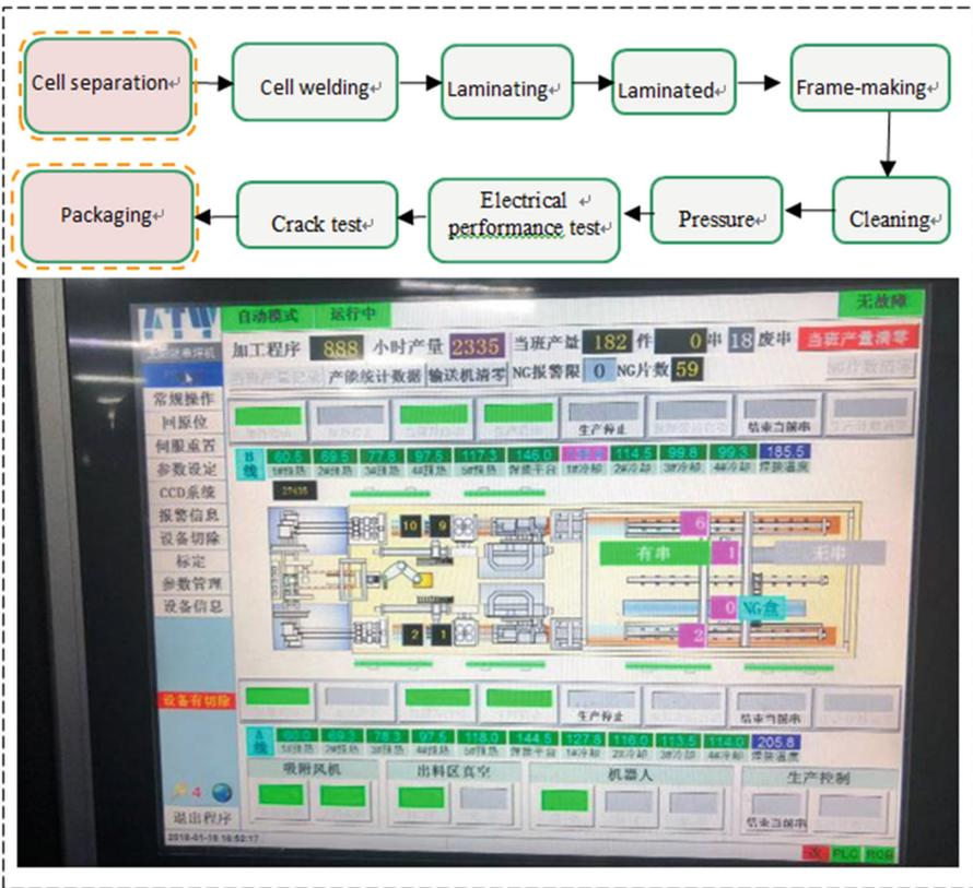
Fig. 3. Control process (above) and visual information interface (following) of photovoltaic modules production line
