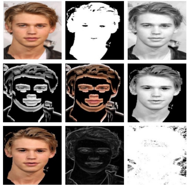
Fig. 2. Some examples from preprocessed image to extract features. (The first image is the colour image. The second image only extracts the regions from skin colours. The third image is the image with only luminosity of different surfaces extracted. The 4,5th images only contain the features, luminosity or colour, around the detected edges. The following two images extract luminosity and colour in the skin-colour area and the last two images were applied with Range and Standard Deviation Texture filters respectively.)
