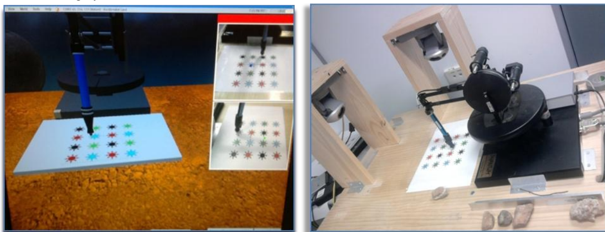
Fig. 3. Teleoperation User Interface using Second Life Interface and Remote Location
