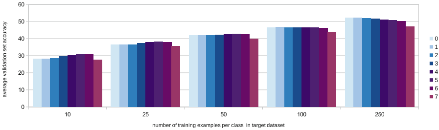
Fig. 5. Number of frozen pre-trained layers. The effect on performance of the number of pre-trained layers of weights frozen during fine-tuning are shown across various target dataset sizes.
