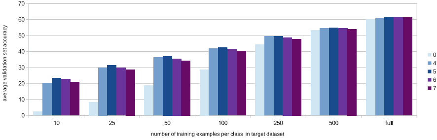
Fig. 1. Number of layers transferred vs dataset size. Each bar represents the average accuracy over the validation set for a model fine-tuned on one size of target training dataset with a particular number of layers of pre-trained weights transferred.
