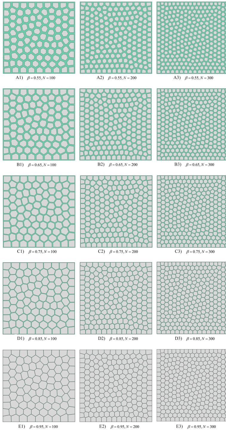
FIG. 5. 15 different foam structures created by the present shrinking algorithm.
