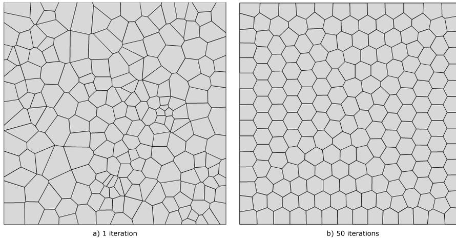
FIG. 2. Schematic diagram of centroid Voronoi tessellations in a square domain with different number of iterations.
