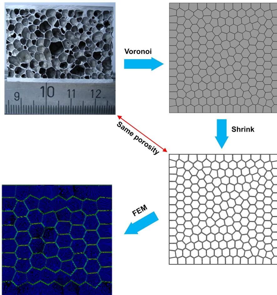
FIG. 1. The basic reconstruction process with shrunk Voronoi tessellations.
