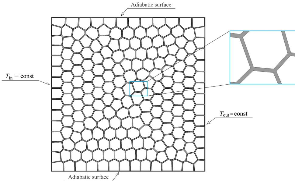
FIG. 4. Example of the generated closed-cell foam structure and the corresponding boundary conditions for heat transfer analysis.
