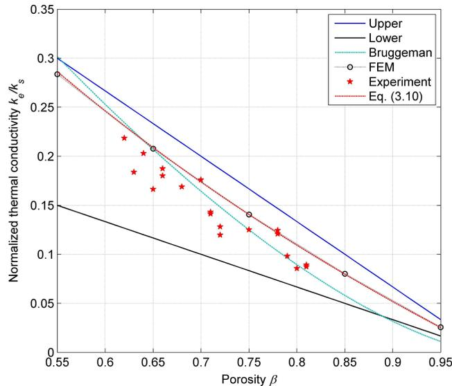
FIG. 7. Comparison of numerical results and other available solutions.
