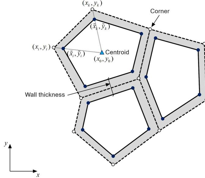
FIG. 3. Schematic diagram of shrinkage of a particular Voronoi polygonal cell.
