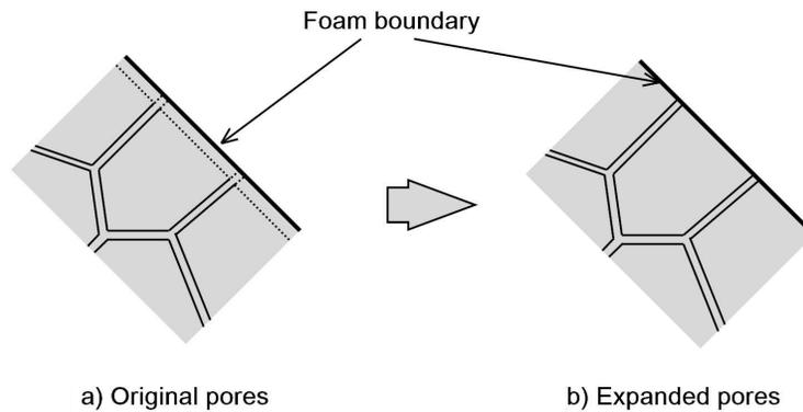
FIG. 6. Expanding procedure for producing open boundary pores.
