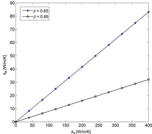
FIG. 8. Variation of the effective thermal conductivity of the foam with that of the solid matrix phase.
