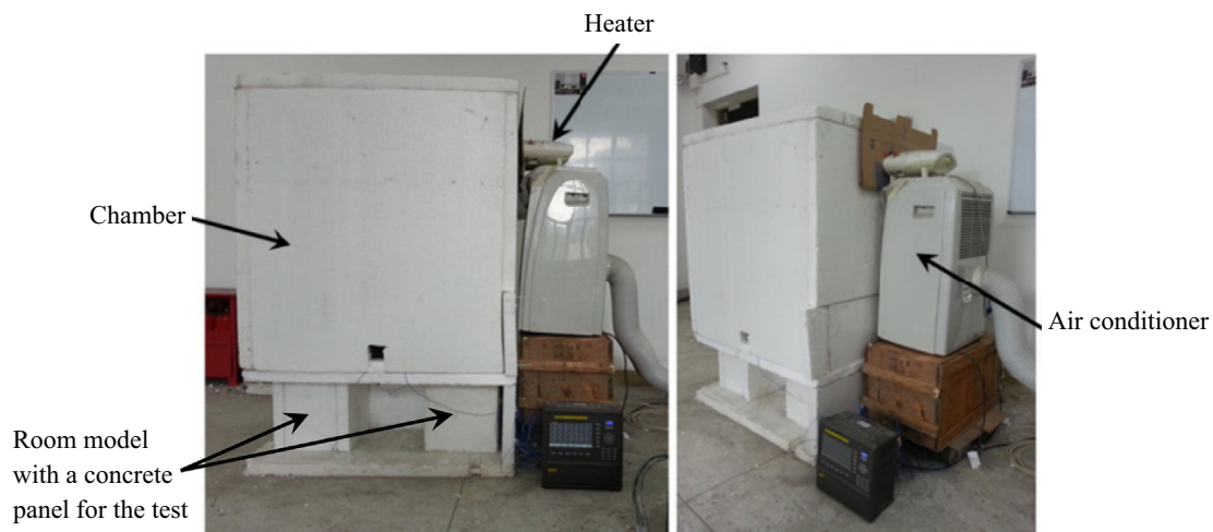
b) Self-designed environmental chamber with heater and air conditioner
