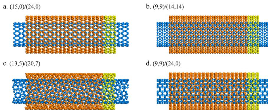
**Figure 1.** Simulation modes of four different DWCNTs with open ends, the atoms (yellow parts) near the right-hand end of the outer tube being fixed.
