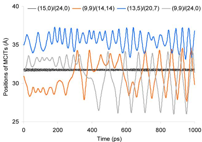
**Figure 4.** Histories of position of mass center of inner tubes (MCITs) in simulation.
