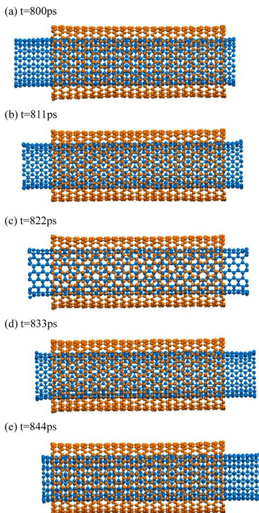
**Figure 6.** Configurations of model (9,9)/(24,0) from 800 to 844 ps (the ends of both walls protrude outward).
