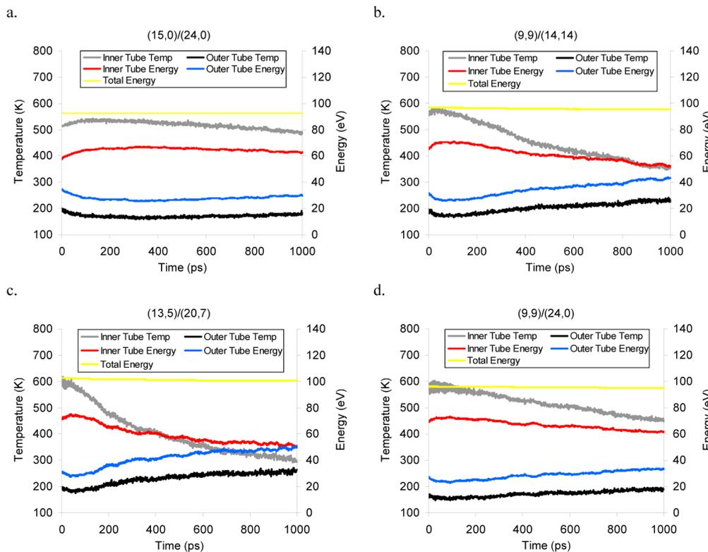
**Figure 3.** Transition histories of temperature and energy (including kinetic energy and potential energy) of bitubes; gray line represents the temperature of the inner tube; black line the temperature of the outer tube; red line the energy of the inner tube; blue line the energy of the outer tube; and yellow line the total energy of the system.
