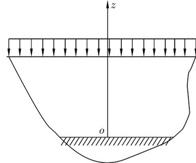
Fig. 2 Uniaxial strain state model.
