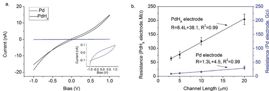
**Fig. 2** Protonic conductivities of the devices with different electrode contacts. (a) Measured protonic current as a function of the voltage bias for the devices with Pd (blue line and insert) and PdH<sub>x</sub> (black line) electrodes. (The channel length was fixed at 3 μm). (b) Measured resistance as a function of the channel length for devices with Pd and PdH<sub>x</sub> electrode contacts.
