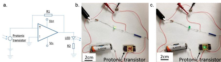
**Fig. 4** The demonstration of a light switch using our optically gated protonic transistor. (a) Schematic drawing of the electrical circuit. (b) Light emitting diode (LED) was on when the illumination light was off. (c) LED was turned off when the illumination light was shone onto the device.
