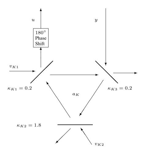
Controller, specified to be quantum, realized as a cavity.
