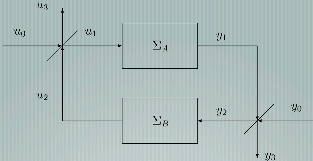
The [small gain theorem](#) asserts stability of the feedback loop if the loop gain is less than one:
