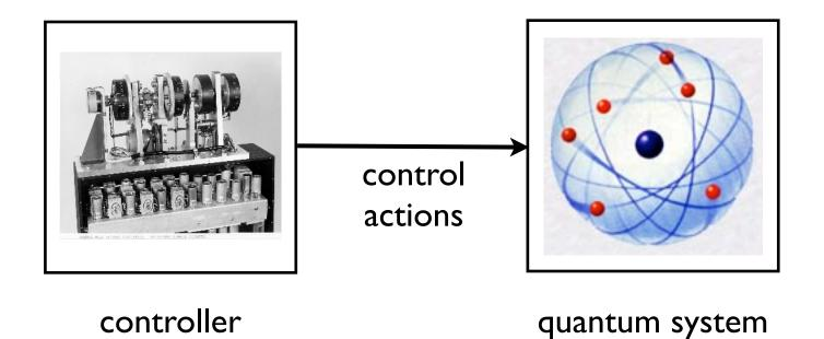
• <u>Closed loop</u> - control actions depend on information gained as the system is operating.
