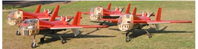
Fig. 3. The four flight vehicles: MK3-Brumby. Four sets of identical GNC modules are installed on the vehicles with different mission load.
