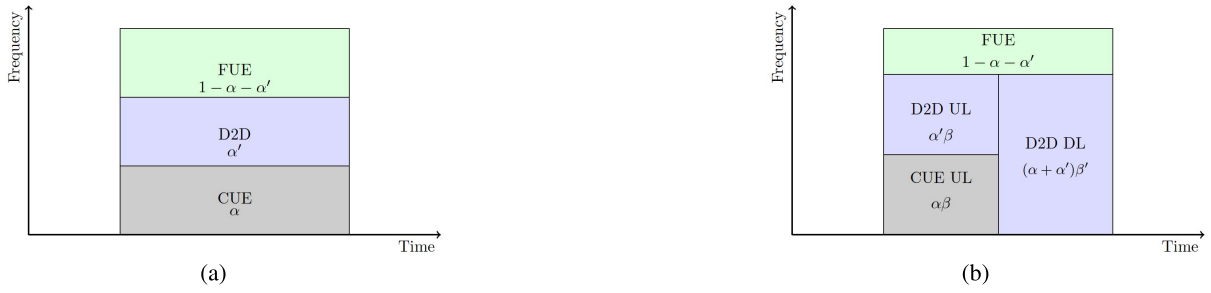
Fig. 4. Illustration of resource allocation in dedicated and cellular modes. (a) Frequency sharing in dedicated mode. (b) Frequency sharing in cellular mode.
