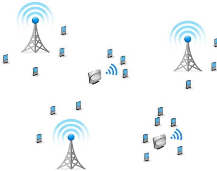
Figure 1.2: HetNets will consist of macro base stations as well as small cells.
