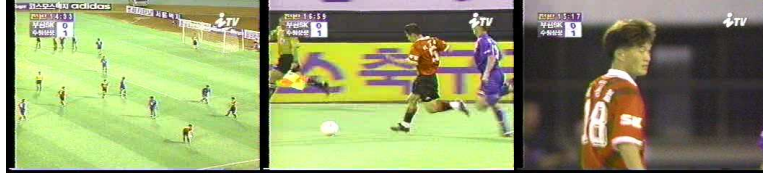
Figure 6.1: Dominant color ratio as an effective feature in distinguishing three kinds of views in soccer video. Left to right: global, zoom-in, close-up. Global view has the largest grass area, zoom-in has less, and close-ups has hardly any (including cutaways and other shots irrelevant to the game).
