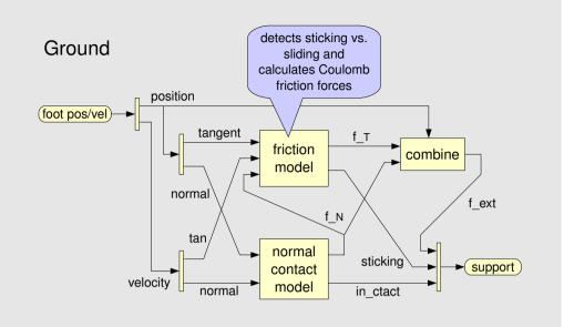
calculates ground Ground reaction forces from normal and tangent components position (foot pos/vel) tangent friction combine model norma f ext normal sticking (support) contact velocity model in ctact
