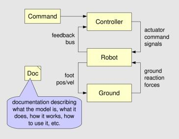
Top-Level Model content depends on what the controller can do Command Controller actuator feedback command bus signals Robot ground Doc foot reaction pos/vel forces Ground
