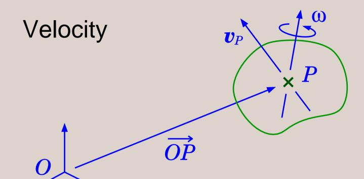
Now introduce a coordinate frame with an origin at any fixed point *O*
