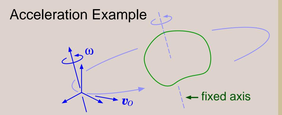
If a body rotates with constant angular velocity about a fixed axis, then its spatial velocity is constant and its spatial acceleration is zero; but each body–fixed point is following a circular path, and is therefore accelerating.
