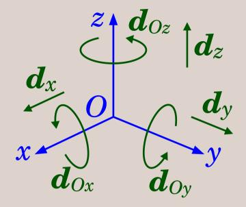
$d_{Ox}$  unit angular motion about the line Ox  $d_{Oy}$  unit angular motion about the line Oy  $d_{Oz}$  unit angular motion about the line Oz
