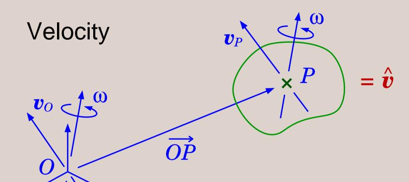
This single quantity provides a complete description of the velocity of a rigid body, and it is invariant with respect to the location of the coordinate frame
