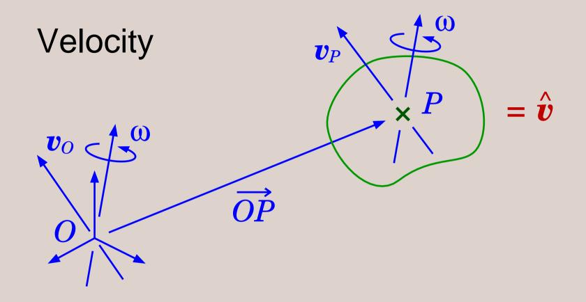
The six scalars  $\omega_x$ ,  $\omega_y$ ,...,  $v_{Oz}$  are the *Plücker* coordinates of  $\hat{\boldsymbol{v}}$  in the coordinate system defined by the frame Oxyz
