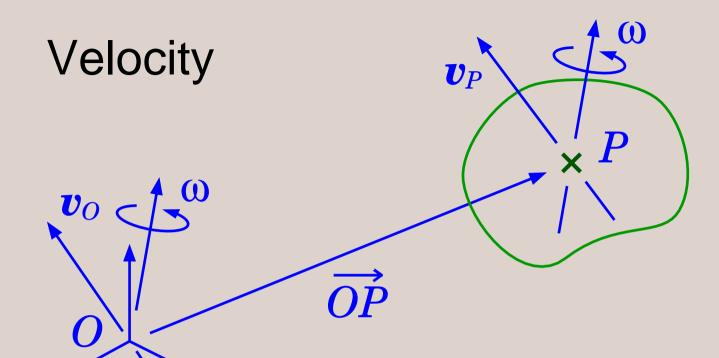
The body can now be regarded as translating with a velocity of  $\boldsymbol{v}_{\mathcal{O}}$  while simultaneously rotating with an angular velocity of  $\boldsymbol{\omega}$  about an axis passing through  $\boldsymbol{\mathcal{O}}$
