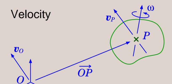
Define **v**<sub>O</sub> to be the velocity of the body–fixed point that coincides with *O* at the current instant
