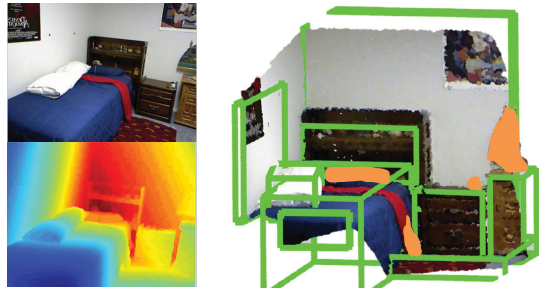
Figure 1: With a given RGBD image (left column), our method explores the 3D structures in an indoor scene and estimates their geometry using cuboids (right image). It also identifies cluttered/unorganized regions in a scene (shown in orange) which can be of interest for tasks such as robot grasping.
