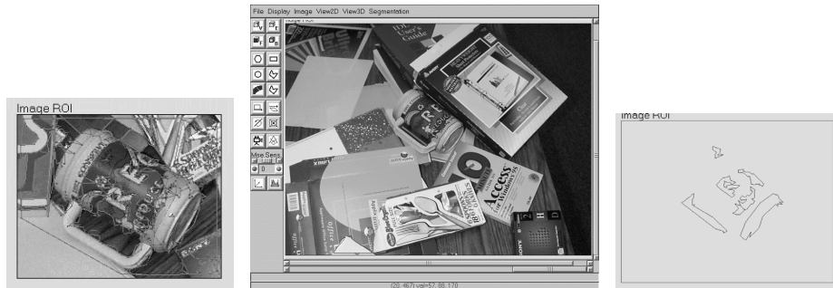
Fig. 9. Recognition of cup image. On the left is the template, in the center the search image and on the right the identified regions of the located cup. Note that the cup in the search image is seen from a different angle from the template image. The letters REC are visible in the template, but only RE is visible in the search image.
