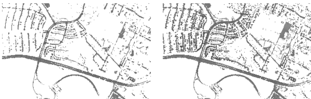
Figure 8: This figure shows the trade-off between using a 1-dimensional (left) or a 2-dimensional (right) linear subspace to identify road pixels. The 2-dimensional classifier allows more natural and lighting variability of the pixel color. This has the effect of picking up more slightly differently colored road regions, while at the same allowing other non-road pixels to be wrongly classified.
