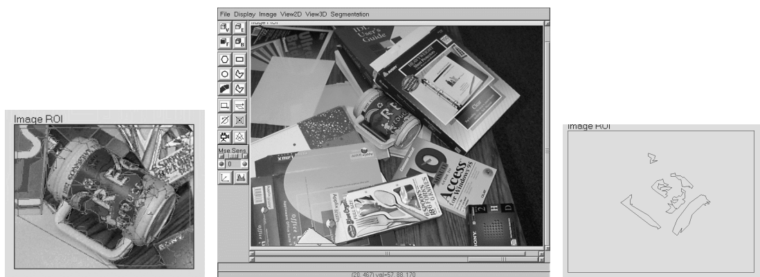
Figure 6: Recognition of cup image. On the left is the template, in the center the search image and on the right the identified regions of the located cup. Note that the cup in the search image is seen from a different angle from the template image.
