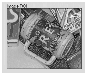
Figure 1: The result of edge detection in a template image containing a cup.
