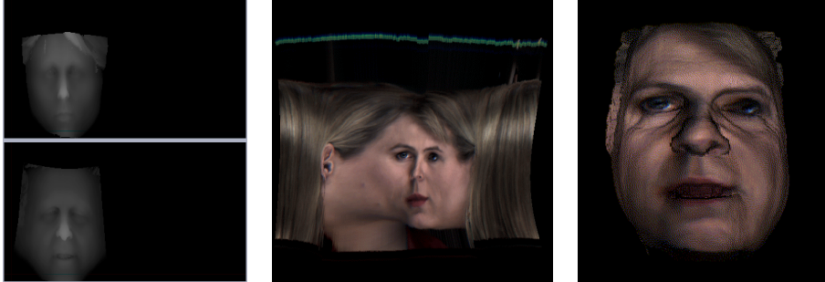
Figure 15: This figure illustrates a mechanism for transferring texture maps. The top left image is the donor face. The bottom left image is the subject face. The middle image is a texture map of the donor face. The right image is the subject face with the donor texture map.
