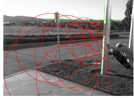
Figure 7: In this image, the apex is unknown, but is constrained to lie somewhere along the vertical direction shown in the image (green). The principal point has two degrees of freedom, but once a position of the principal point is assumed, the focal length of the camera may be computed. The red circles represent various estimates of the focal length for different assumed principal points. Each circle is the locus of all directions 10^\circ from the principal point, which is at the centre of the circle. Thus, the radius of each circle is equal to 0.176f = \tan(10^\circ)f . The focal length has been computed in each case using (2).
