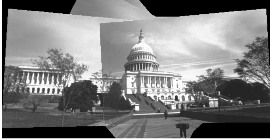
Fig. 1. A composite image constructed from five different views of the Capitol. The composite image shows very clearly the projective distortion necessary for matching the images. Analysis of this projective distortion provides the basis for the calibration algorithm.
