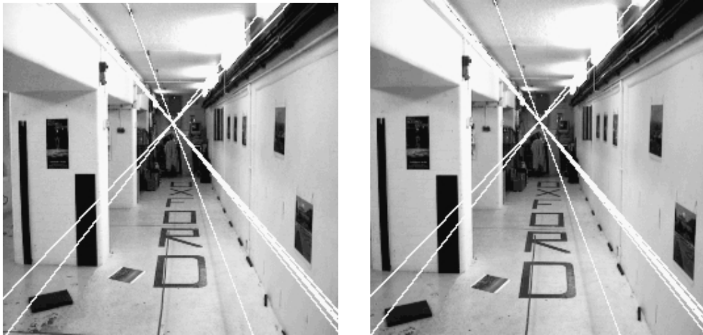
Figure 2.4: Corridor Scene In the corridor scene the epipoles are right in the image.
