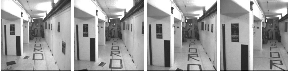
Fig. 4. Image sequence II: four images from a nine image sequence. Planar motion with the rotation axis approximately aligned with the image y axis. 75 corners are automatically matched across the 9 images. The sequence was acquired by a camera mounted on an AGV.
