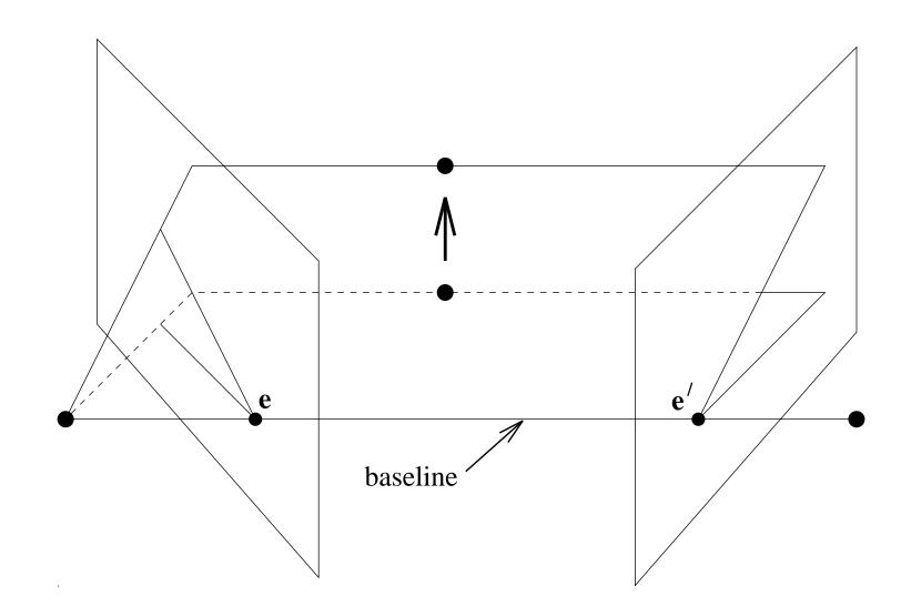
As the position of the 3D point  $\mathbf{X}$  varies, the epipolar planes "rotate" about the baseline. This family of planes is known as an epipolar pencil. All epipolar lines intersect at the epipole.
