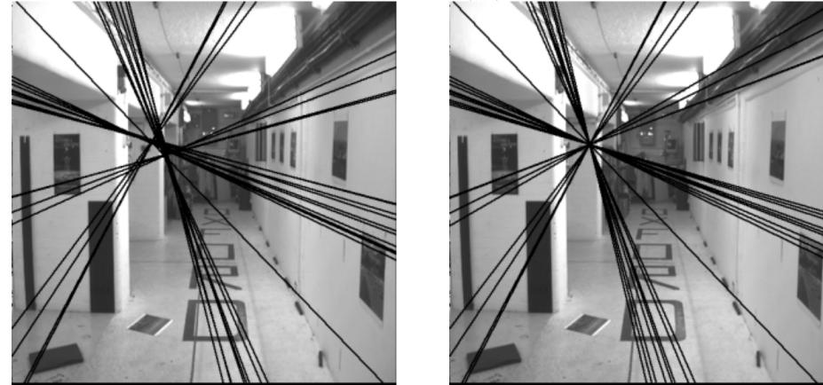
Left: Uncorrected F – epipolar lines are not coincident.
