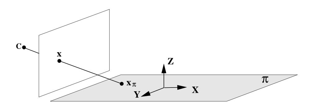
Choose the world coordinate system such that the plane of the points has zero z coordinate. Then the  $3 \times 4$  matrix P reduces to
