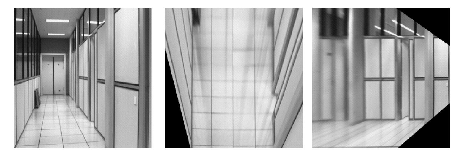
The synthetic images are produced by projectively warping the original image so that four corners of an imaged rectangle map to the corners of a rectangle. Both warpings correspond to a synthetic rotation of the camera about the (fixed) camera centre.
