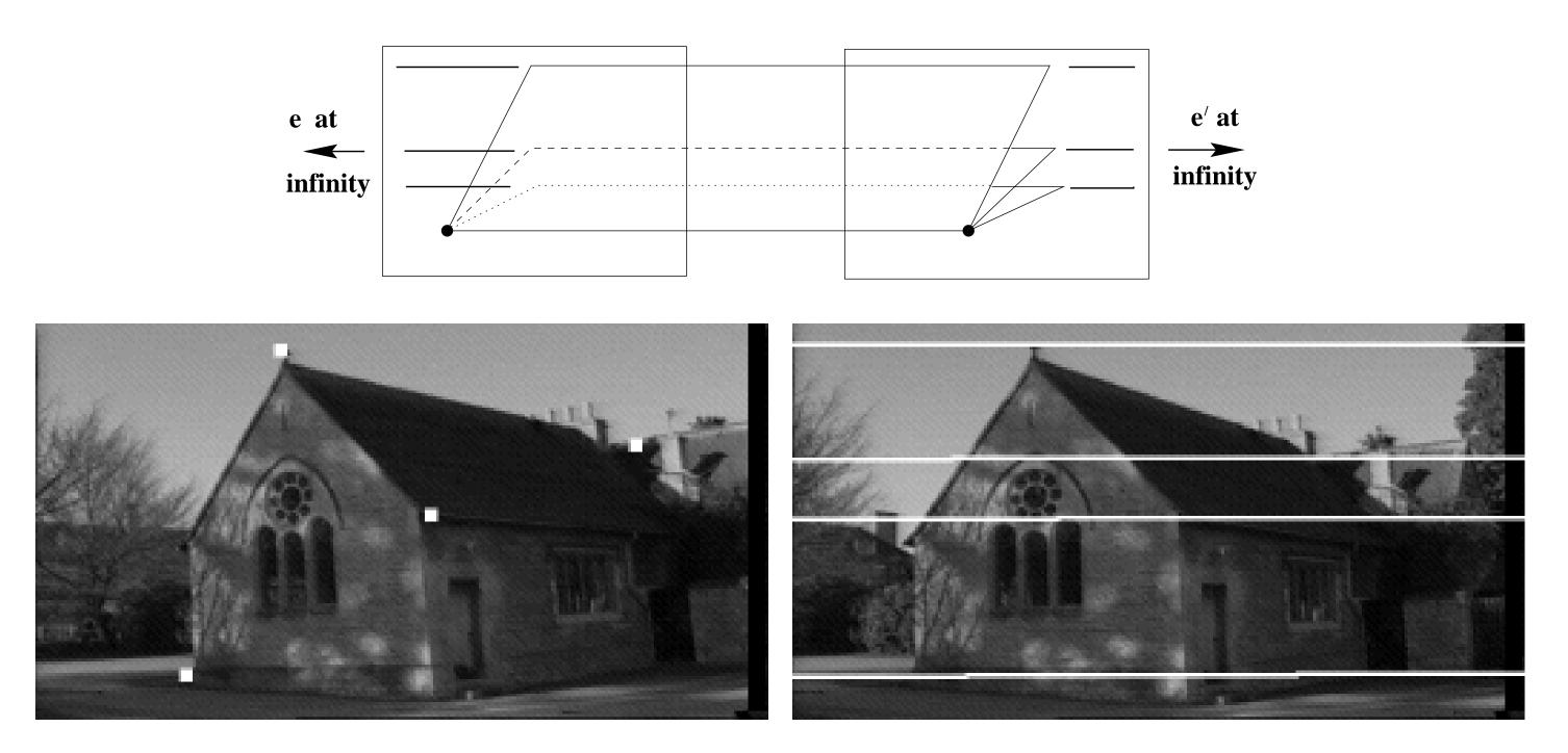
Epipolar geometry depends only on the relative pose (position and orientation) and internal parameters of the two cameras, i.e. the position of the camera centres and image planes. It does not depend on structure (3D points external to the camera).
