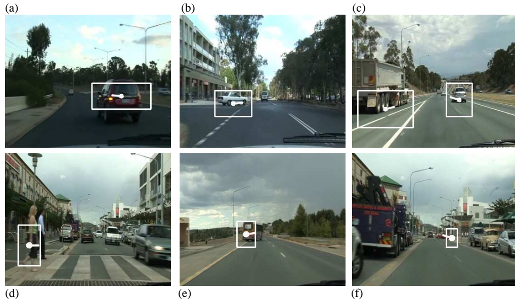
Figure 9.3: Sample hazard detections from video segment (vs) testing: (a) merge from right (vs 1, 29.36 sec), (b) car turns out from left (vs 1, 52.79 sec), (c) truck merges from left (vs 1, 271.45 sec), (d) pedestrians crossing (vs 5, 101.78 sec), (e) bus pulls out from left (vs 6, 166.93 sec), (f) car crosses road from right (vs 5, 109.84 sec)
