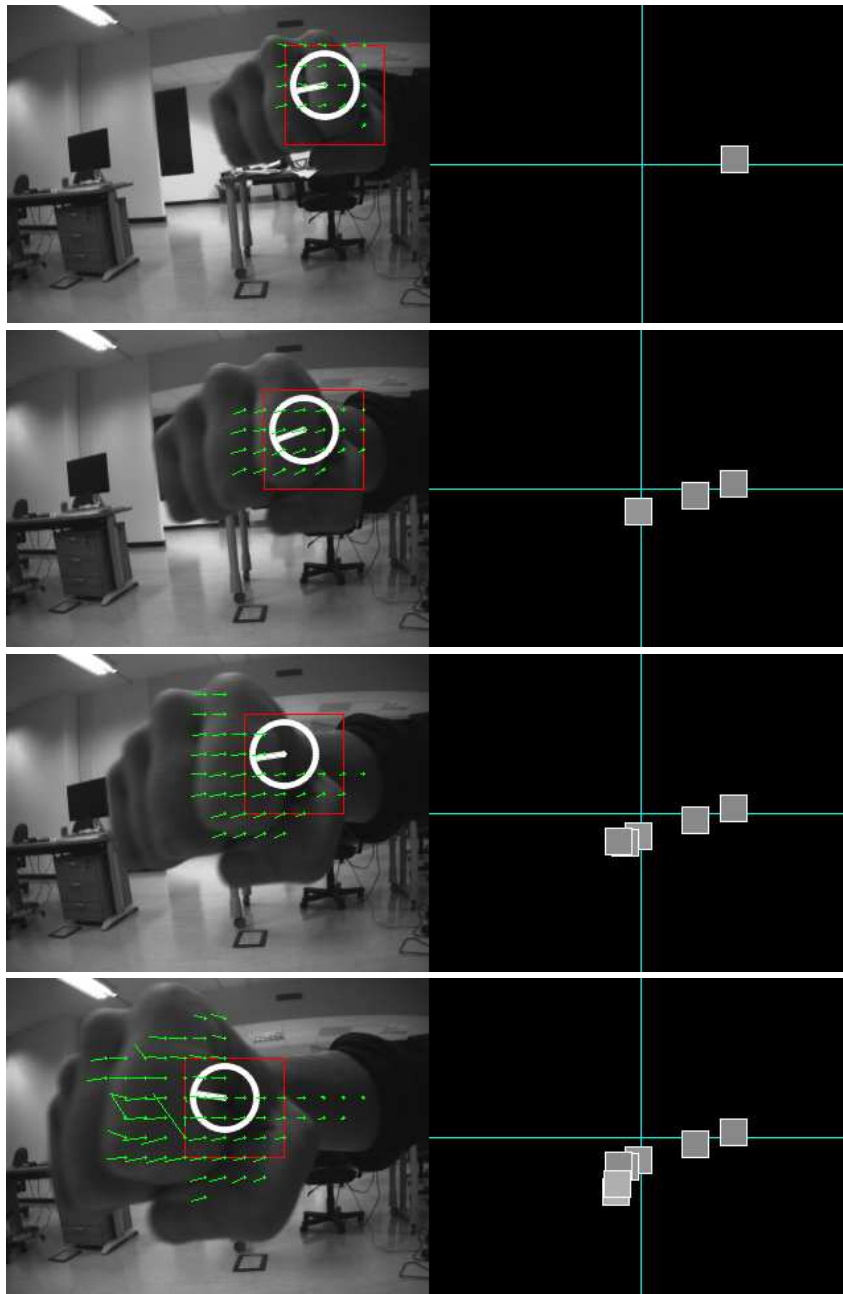
Figure 8.8: Sample output frames from live impact prediction test for an incoming closed fist. Left image shows the optical flow in the segmented region of motion, and the estimated direction of translational motion in the plane. The red box represents the region of maximum divergence. Right image shows estimated location of impact about the camera. Increasing brightness in impact markers represents the estimated time-to-contact. Complete output from the impact prediction algorithm is given in Video 8.1 of the supplementary CD-ROM to this thesis.
