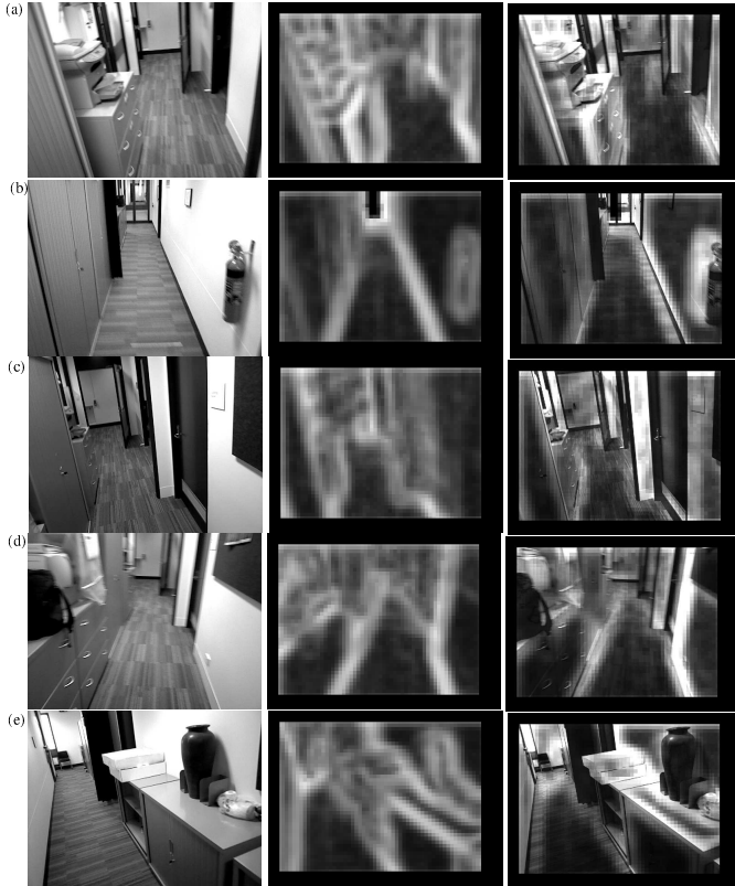
Fig. 1. Example frames from the office data set showing from left to right: the original image, the estimated perturbation map and the resulting augmented intensity image.
